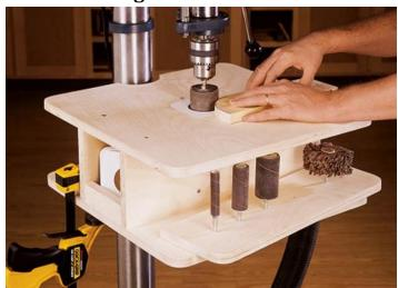
This handy table helps you in three important ways. First, it has a dust-collection port for capturing fine dust before it becomes airborne. The table also accepts inserts that you size to tightly fit your sanding drums. That provides workpiece support and improves dust-collection efficiency. And, with storage areas for sanding drums and inserts, you'll always be organized.
